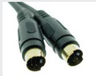
3-2: A single S-Video cable is actually several cables in one. That's because the S-Video format separates brightness and color information before sending it through a multi-conductor cable.
